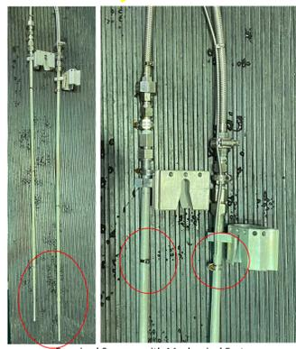
Repaired Sensors with Mechanical Fasteners
