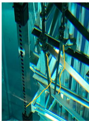
Sensors with Damaged Capillary Tubes
